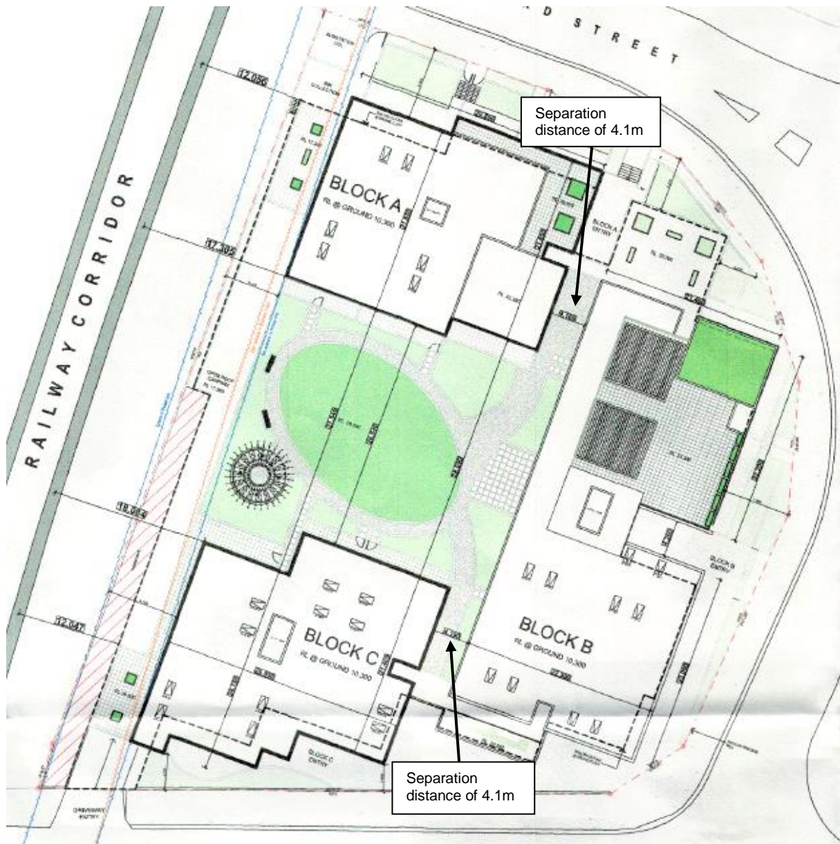
Figure 18: Extract of the site plan demonstrating the non-compliant building separation distances.
